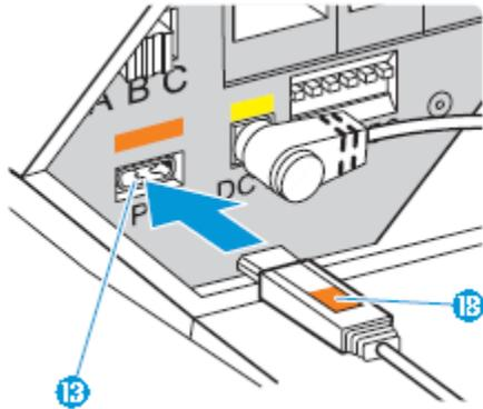
3. Complete the set-up as shown in the Quick Guide, by activating the connection, setting the slider switch (A,B,C) to the position that allows you to hear a dial tone, and then make a call and set the outgoing microphone volume on the rotary switch while a person on the other end of the call gives you feedback on volume while you talk. See figure below.
