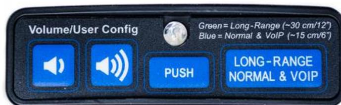
1. **Microphone "Push" Button:** The "Push" button controls the on/off behavior of the microphone and can be set to work in one of three modes:
